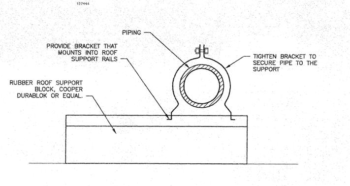
PIPING ROOF SUPPORT DETAIL M402 SCALE: N.T.S.
