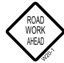
Sign on Type II Barricade 200' from work zone
