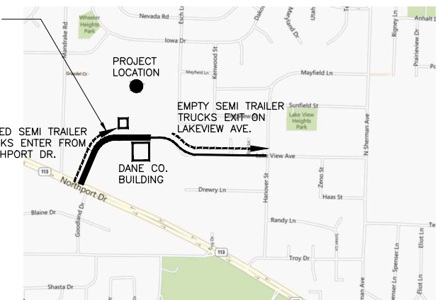
CONTRACTOR SEMI TRAILER TRUCK ROUTE ACCESS PLAN
