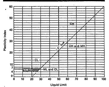
For classification of fine-grained soils and fine fraction of coarsegrained soils.
