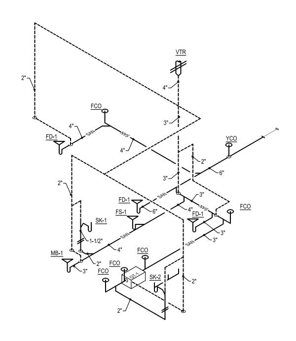
SANITARY WASTE AND VENT RISER DIAGRAM
