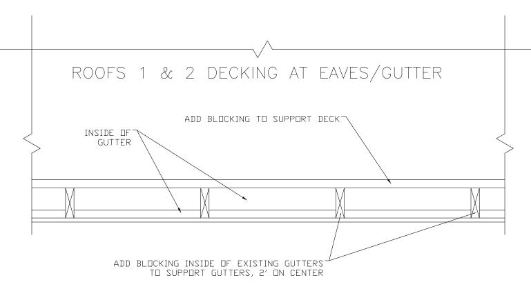
DETAIL A-1.2/01TOP VIEW OF GUTTER BLOCKING FOR ROOFS 1 & 2
