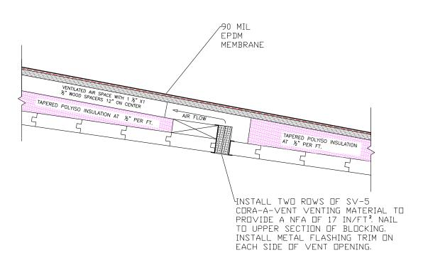
SOFFIT VENTILATION DETAILS FOR ROOFS 3&6
