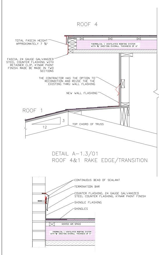
DETAIL A-1.3/04 FLASHING AT CHIMNEY
