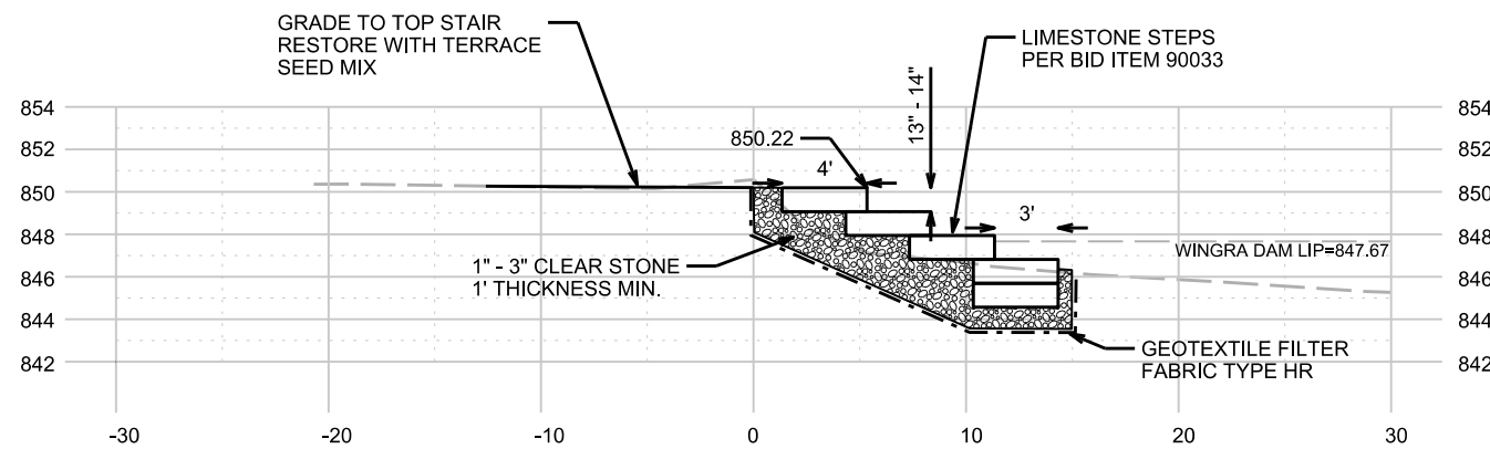
STATION 13+70: DOLOMITIC LIMESTONE STEPS
