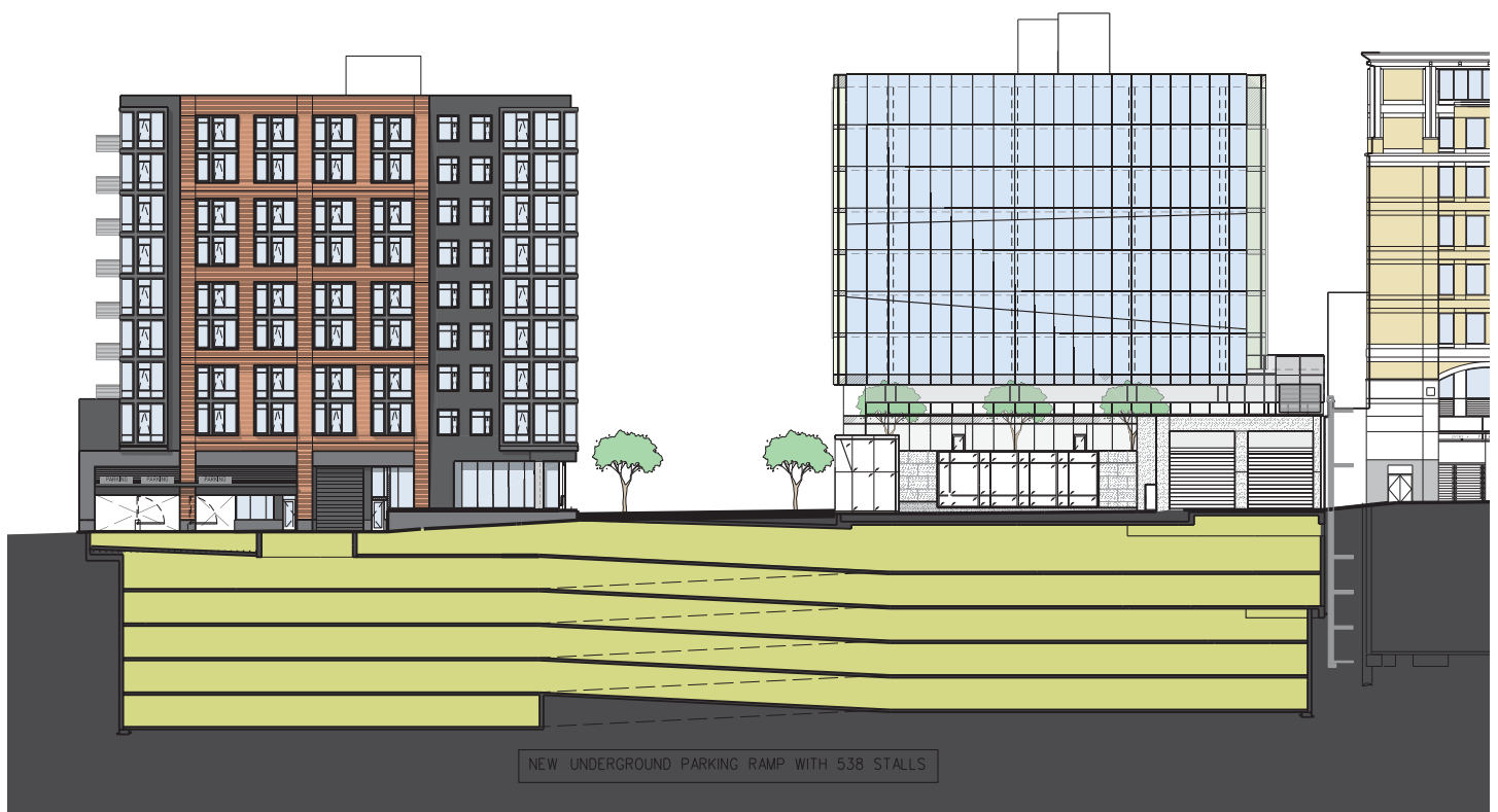
Doty Street section highlighting underground parking at Anchor Properties redevelopment.
