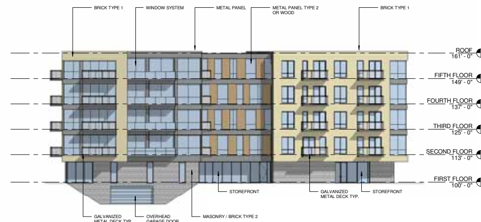
3 OVERALL SOUTH ELEVATION A201 1/16" = 1'-0"
