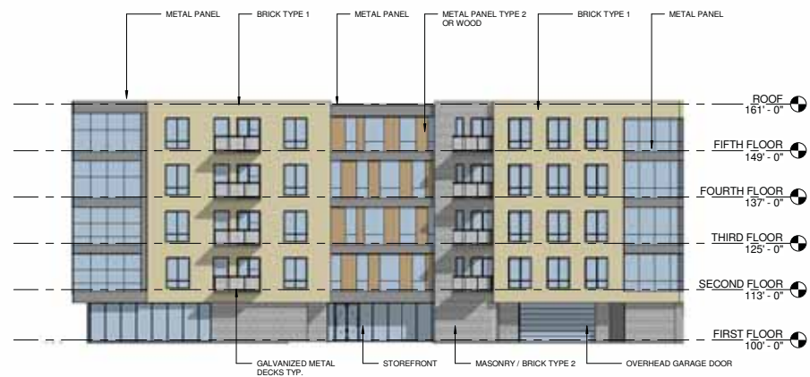
1 OVERALL NORTH ELEVATION - WEST WILSON STREET A201 1/16" = 1'-0"
