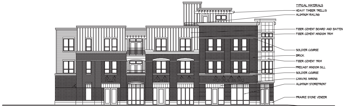
ELEVATION ALONG MONROE STREET 1/8" = 1'-0"
