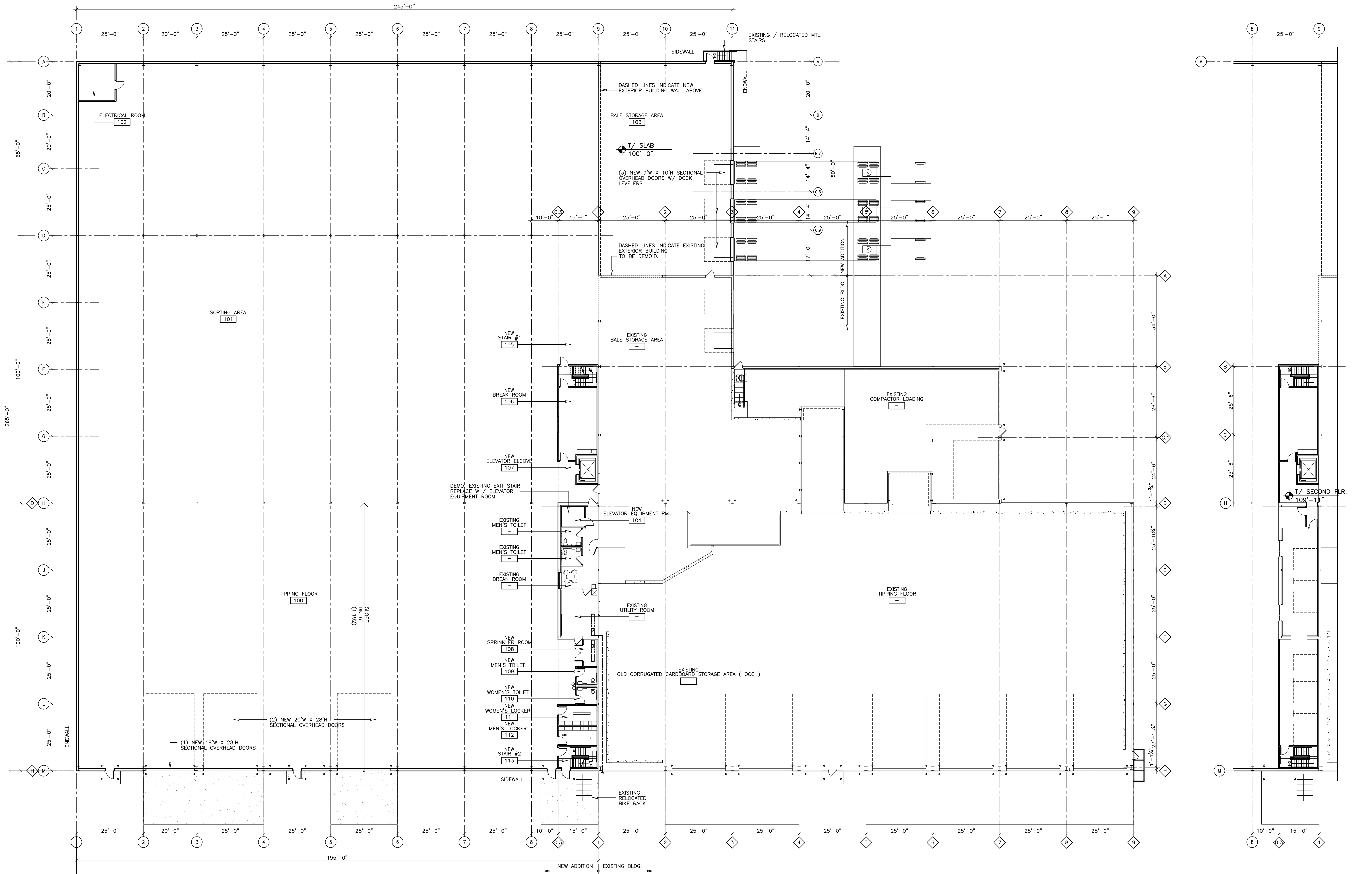
1 FIRST FLOOR PLAN 1/16" = 1'-0" NEW ADDITION 54,946 SQ. FT. EXISTING 30,148 SQ. FT.
