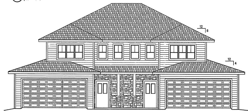
3 ALLEY ELEVATION \frac{3}{16}'' = 1'-0''
