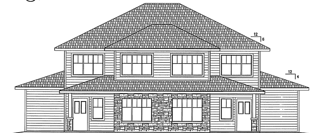
4 STREET ELEVATION - BUILDING "C" & "D" 3/16" = 1'-0"
