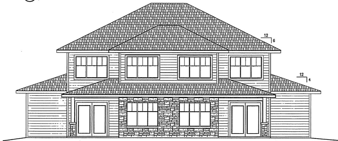
4 STREET ELEVATION - BUILDING "E," "G" & "J" \frac{3}{16}'' = 1'-0''
