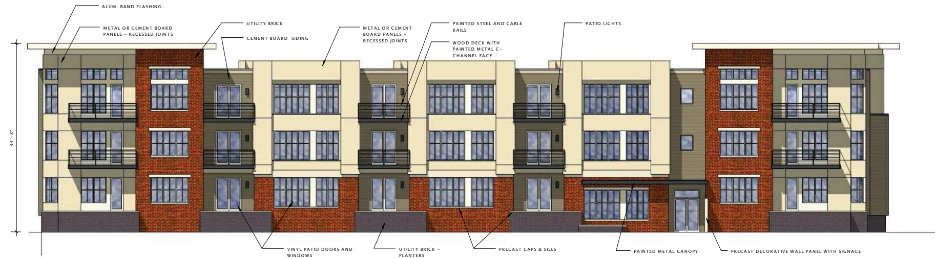
① Building A - Front Elevation 3/32" = 1'-0"
