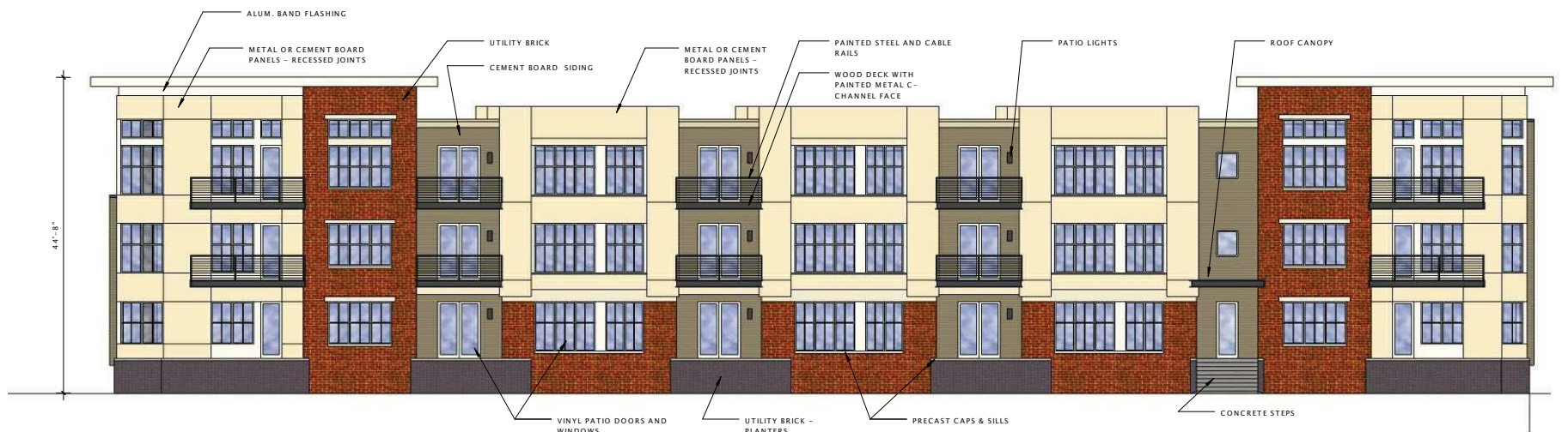
② Building A - Back Elevation 3/32" = 1'-0"
