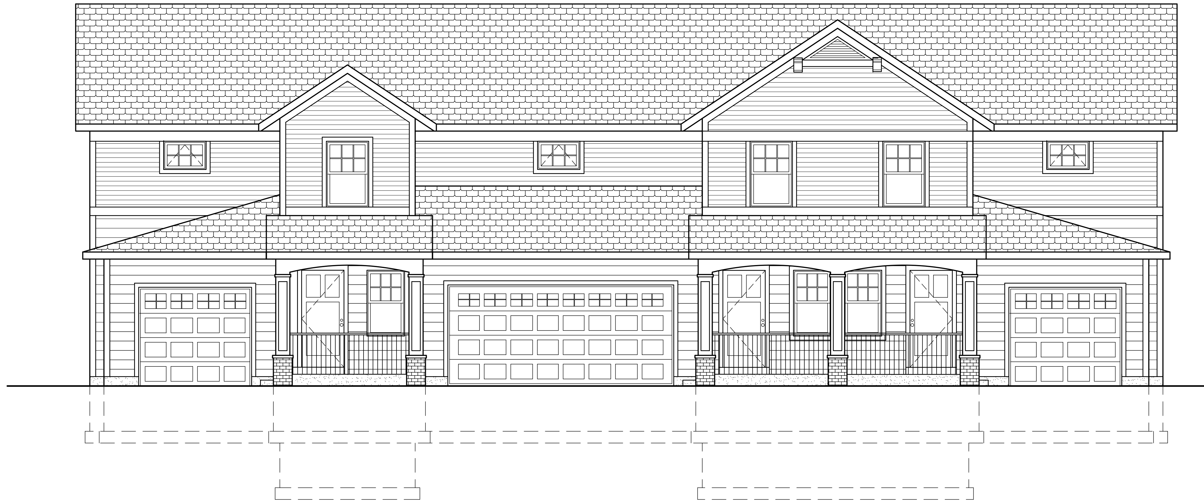
1 EXTERIOR ELEVATION- BLDGS 3,7 SCALE: 1/4"=1'-0"
