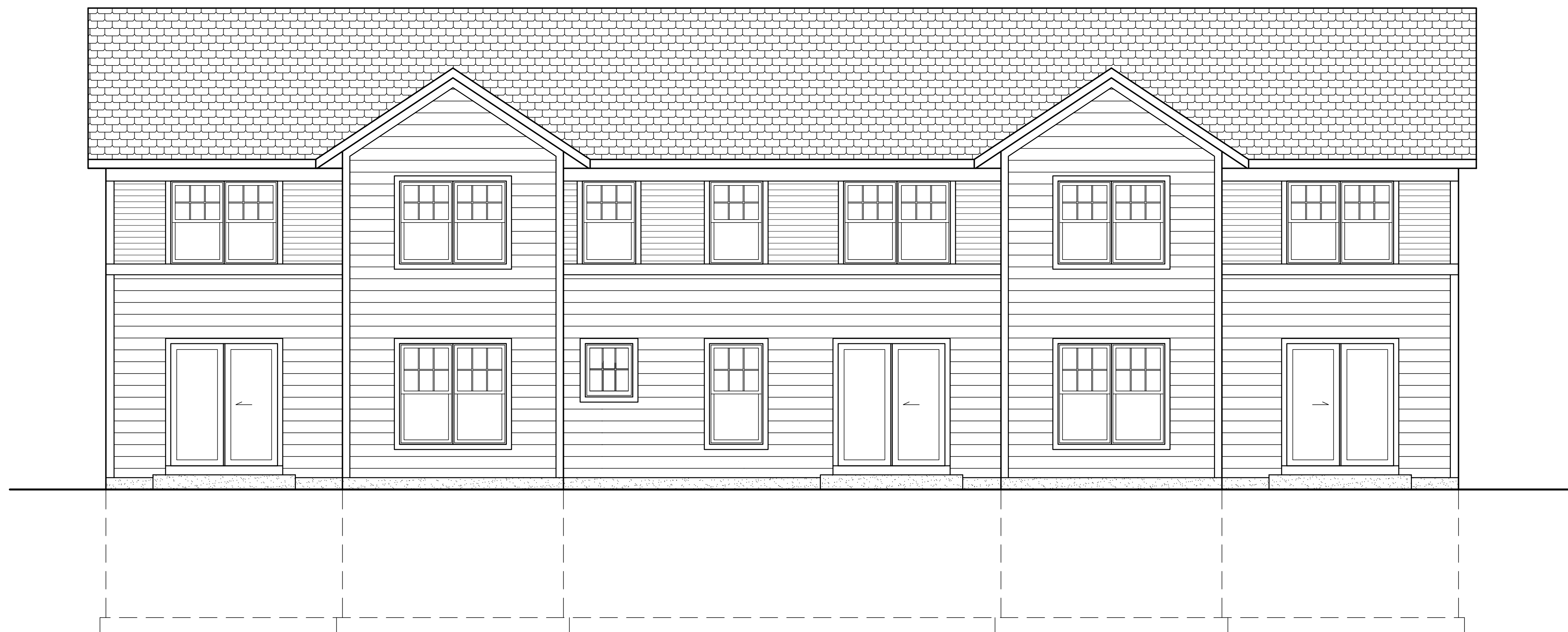
3 EXTERIOR ELEVATION- BLDGS 3,7 SCALE: 1/4"=1'-0"
