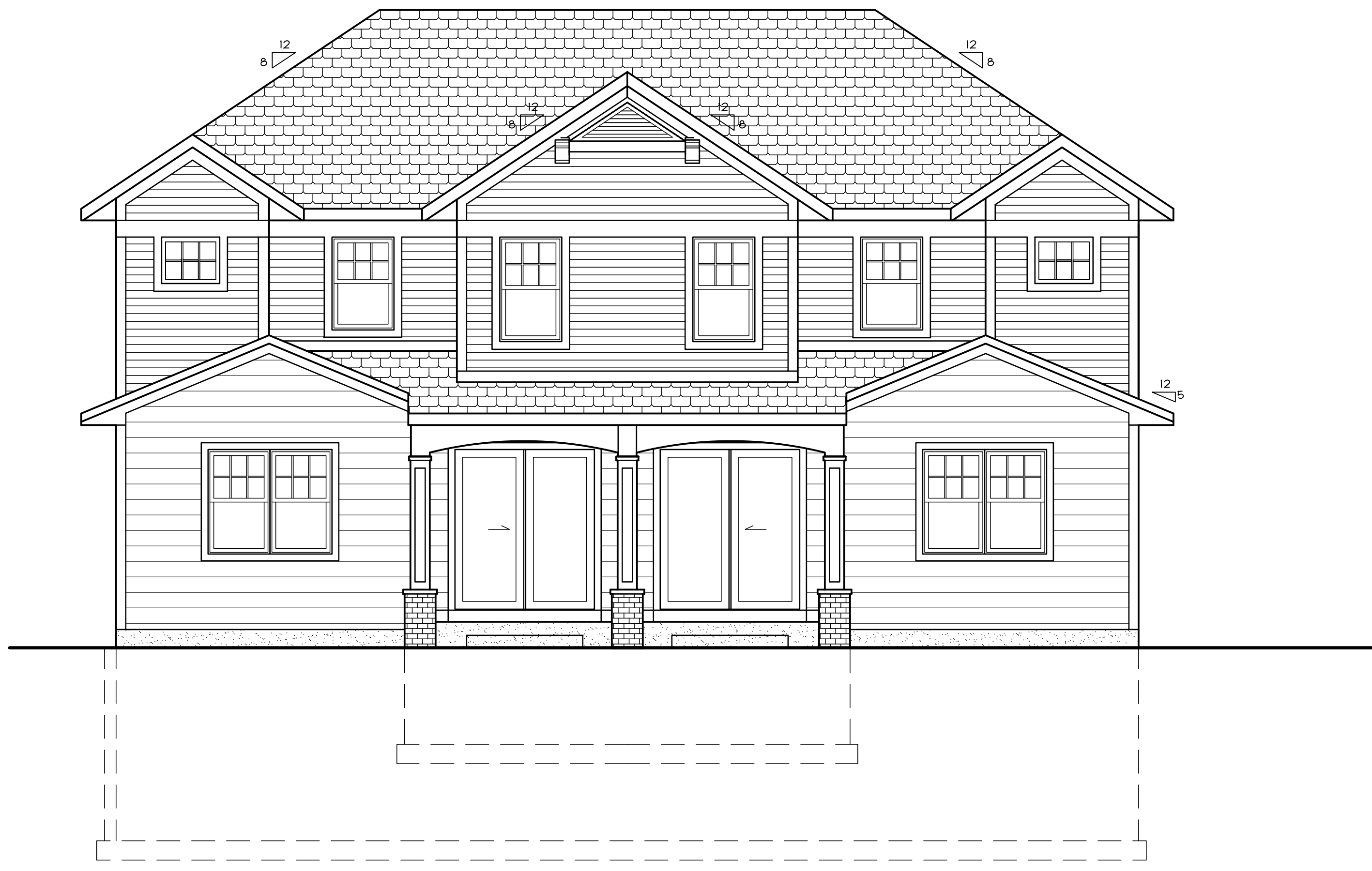
③ REAR EXTERIOR ELEVATION- BLDGS #4,8,10 SCALE: 1/4"=1'-0"
