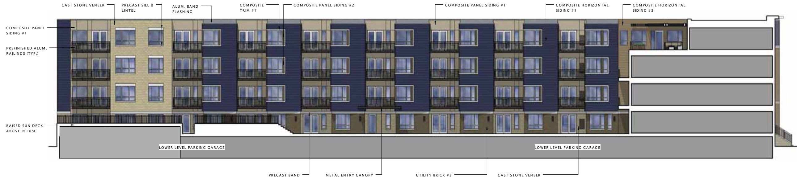
② Interior Courtyard Elevation - North 3/32" = 1'-0"
