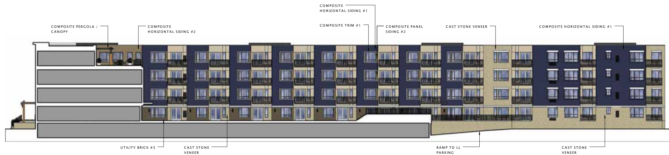
③ Interior Courtyard Elevation - East 1/16" = 1'-0"
