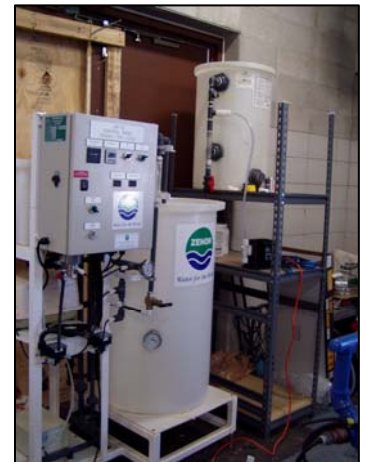
Photo 3: Membrane Pilot System
