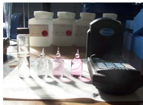
Photo 6: Chlorine Field Test Equipment
