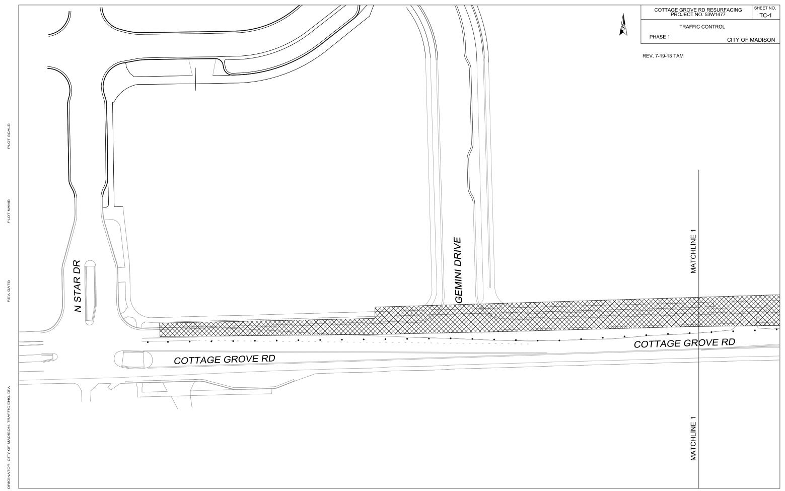
SHEET NO. COTTAGE GROVE RD RESURFACING PROJECT NO. 53W1477 TC-2 TRAFFIC CONTROL PHASE 1 CITY OF MADISON REV. 7-19-13 TAM MATCHLINE 2 MCLEAN DRIVE Minimum width of traffic lane is 10' to edge of pavement — or 12' to face of curb. COTTAGE GROVE RD COTTAGE GROVE RD
