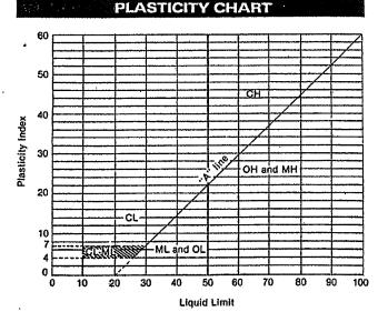
For classification of fine-grained solls and fine fraction of coarsegrained soils.
