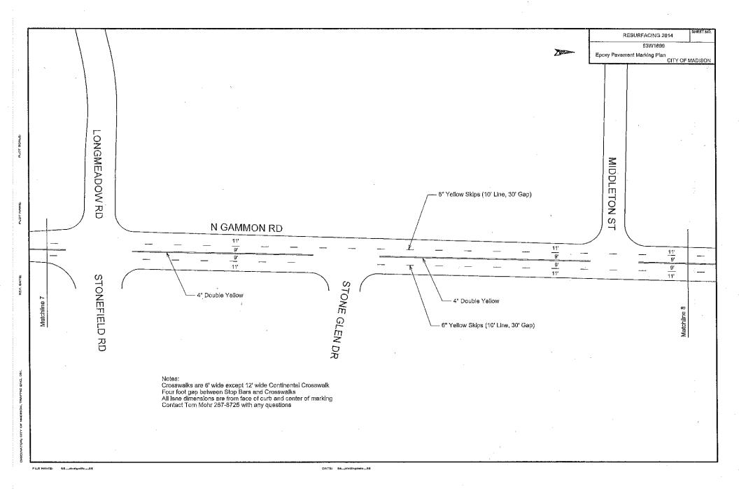
RESURFACING 2014 53W1699 Epoxy Pavement Marking Plan CITY OF MADISON 6" Yellow Skips (10' Line, 30' Gap) N GAMMON RD 11' 9' 11' 4" Double Yellow – 6" Yellow Skips (10' Line, 30' Gap) Notes: Crosswalks are 6' wide except 12' wide Continental Crosswalk Four foot gap between Slop Bars and Crosswalks All lane dimensions are from face of curb and center of marking Contact Tom Mohr 267-8725 with any questions DATE: \$5...plattingdate...\$5 FILE NAME: \$\$....des/gnfile....\$\$
