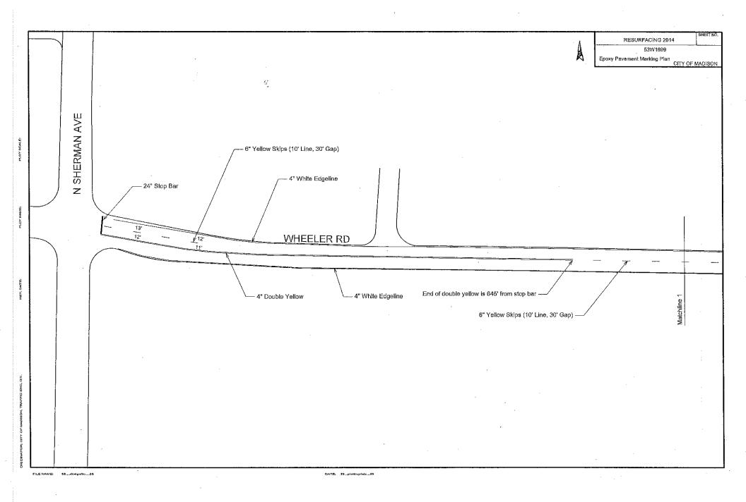
RESURFACING 2014 53W1699 Epoxy Pavement Marking Plan CITY OF MADISON - 4" White Edgeline - 6" Yellow Skips (10' Line, 30' Gap) WHEELER RD Matchline 1 - 4" White Edgeline FILE NAME: \$5....devignfile...55 DATE: \$5...piottingstate...\$5
