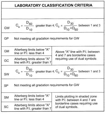
Determine percentages of sand and gravel from grain-size curve. Depending on percentage of fines (fraction smaller than No. 200 sieve size), coarse-grained soils are classified as follows:
