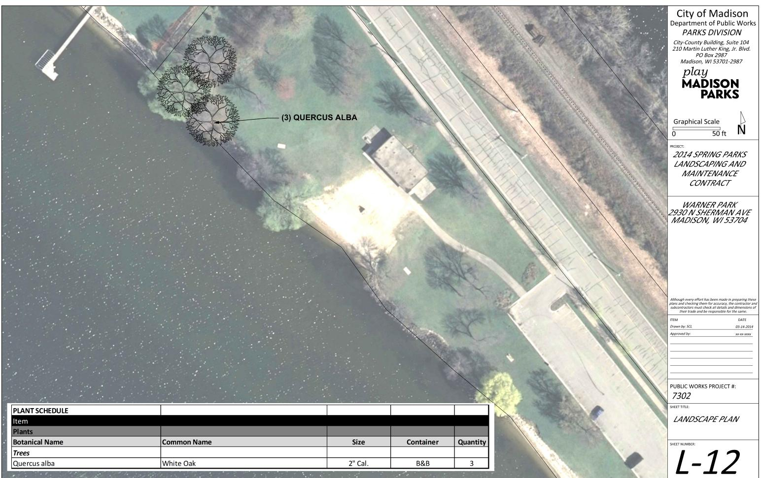
NOTE: 1. THIS TREE WILL REPLACE EXISTING ASH TREE, TO BE REMOVED BY CONTRACTOR. EXACT TREE TO BE REMOVED SHALL BE DETERMINED BY ENGINEER. BID ITEMS 20401 AND 20402 INCLUDE QUANTITY FOR REMOVAL OF 14" I.D. ASH TREE. 2. PROPOSED TREE LOCATION TO BE MARKED IN FIELD BY CITY STAFF TO REPLACE EXISTING ASH TREE.
