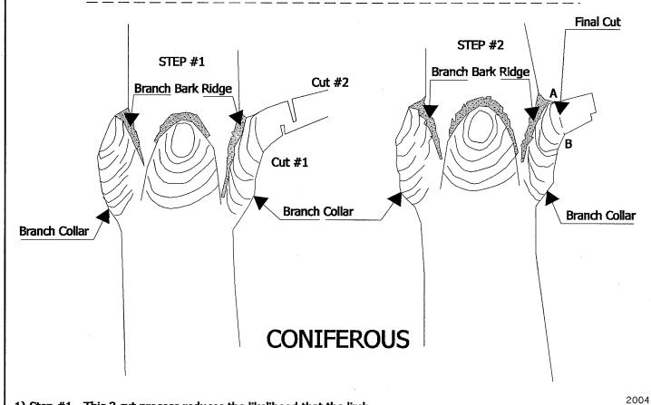
Step #1 - This 2 cut process reduces the likelihood that the limb will peel and cause additional unwanted tissue damage
