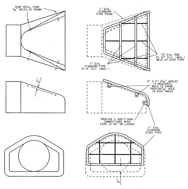
THE CONTRACTOR SHALL BOLT THE PIPE GATE TO THE CONCRETE ENDWALL WITH FOUR  $^{3}8^{\prime\prime}$  X 6  $^{\prime\prime}$  MACHINE BOLTS WITH NUTS ON INSIDE WALL.
