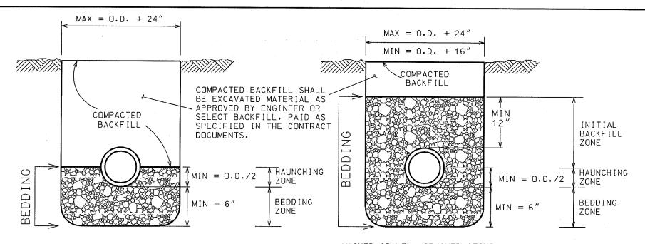
WASHED GRAVEL OR CRUSHED STONE AS SPECIFIED IN SECTION 502.1 (d), BEDDING OF SEWER PIPES
