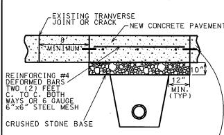
SEE SDD 3.10 FOR DOWEL AND PAVEMENT TIE INSTALLATION
