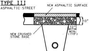
THE PATCH SHALL BE CRUSHED STONE BASE COURSE. GRADATION NO. 2 OVERLAID WITH ASPHALT UPPER LAYER EQUAL IN THICKNESS TO THE EXISTING ASPHALTIC PAVEMENT WITH A MINIMUM THICKNESS OF 3" AND A MAXIMUM THICKNESS OF 51% UNLESS OTHERWISE SPECIFIED AND LAID IN ONE OR MORE COURSES AS DIRECTED BY THE ENGINEER.
