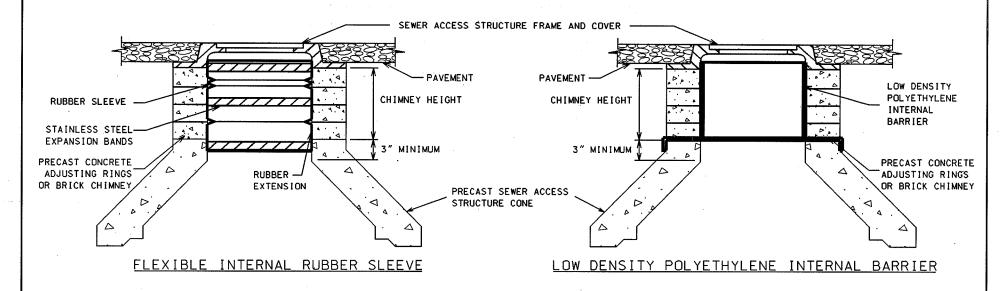
AN INTERNAL CHIMNEY SEAL WHERE NEEDED. SHALL BE INSTALLED TO COVER THE ENTIRE CHIMNEY AREA IN ACCORDANCE WITH THE MANUFACTURER'S INSTRUCTIONS. FRAME SEALS SHALL CONSIST OF ONE OF THE FOLLOWING TYPES OF INTERNAL SEALS:
