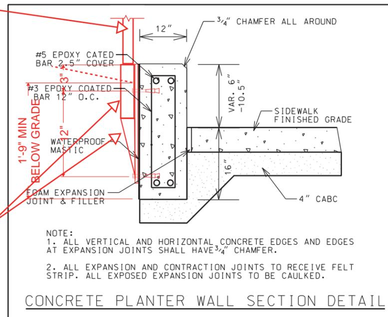
CONCRETE PLANTER WALL SECTION DETAIL
