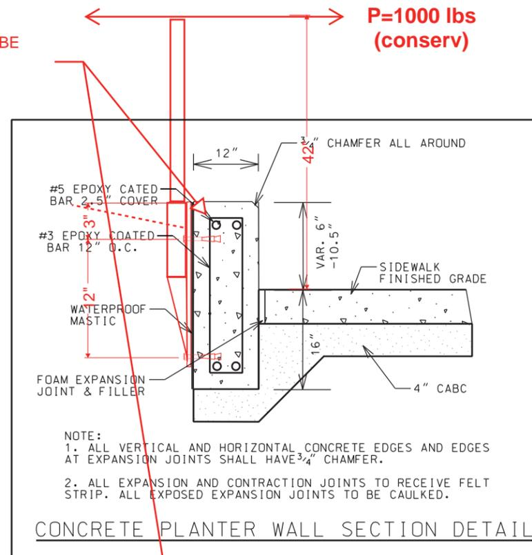
CONCRETE PLANTER WALL SECTION DETAIL
