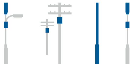
Possible small cell locations, on existing utilities (left), or new freestanding poles (right).
