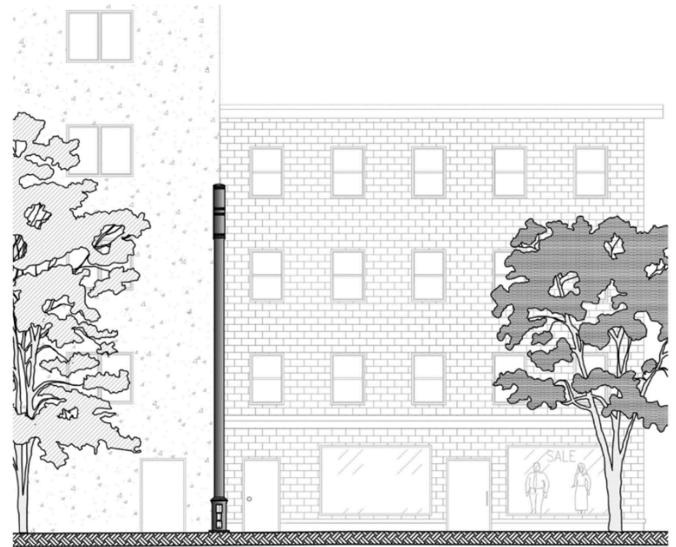
Small Cell in Commercial Area
