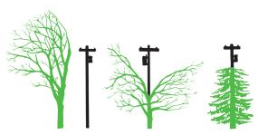
The amount of pruning is based on the type of tree and how close the tree is to the wires. These are examples of pruning according to international pruning standards.
