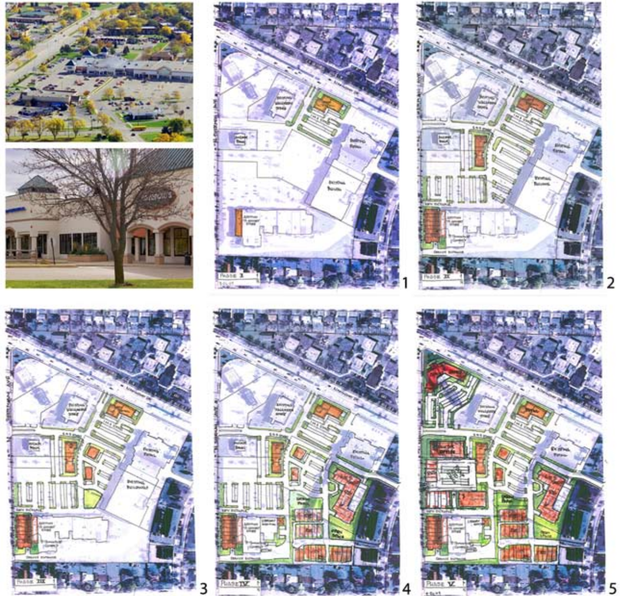
Figure I-5: Potential phasing for redevelopment of the Northside TownCenter. Note: Tear downs and new construction can span 10 or more years. The key is to reserve land for the main street to ensure that the phased construction can eventually achieve the town square concept.
