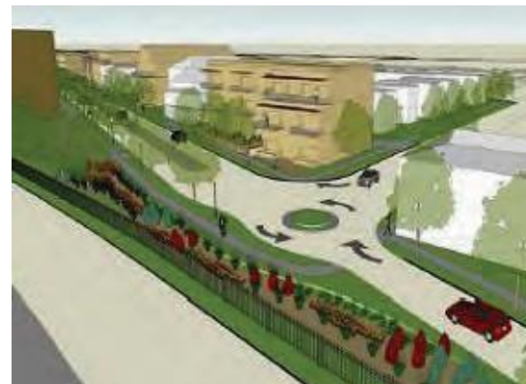
The gateway could be enhanced by installation of a traffic calming measure and a rain garden.
