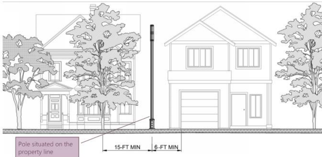
Figure 5-3.2: Freestanding Small Cell Location Between Property and Trees
