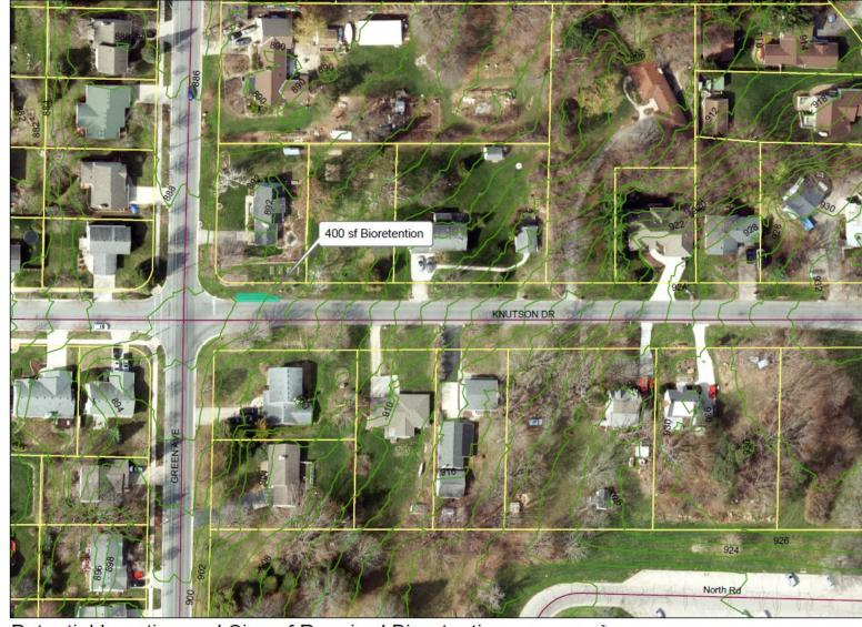
Potential Location and Size of Required Bioretention Knutson Dr.
