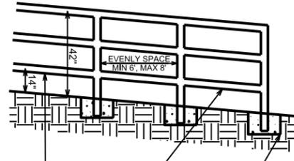
2 1/2" NOMINAL I.D. STANDARD WEIGHT STRUCTURAL STEEL TUBING
