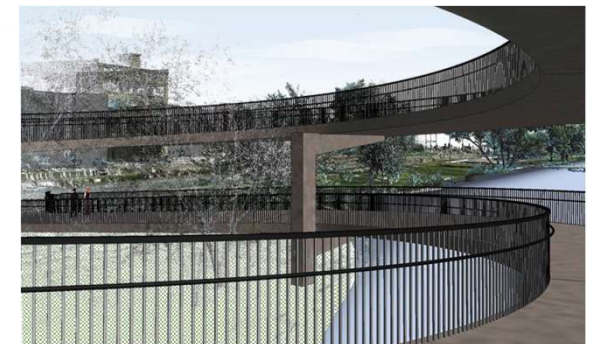
The pier supporting the pedestrian bicycle overpass ramp can be cantilevered, yet some of the structure would still extend over the lake..
