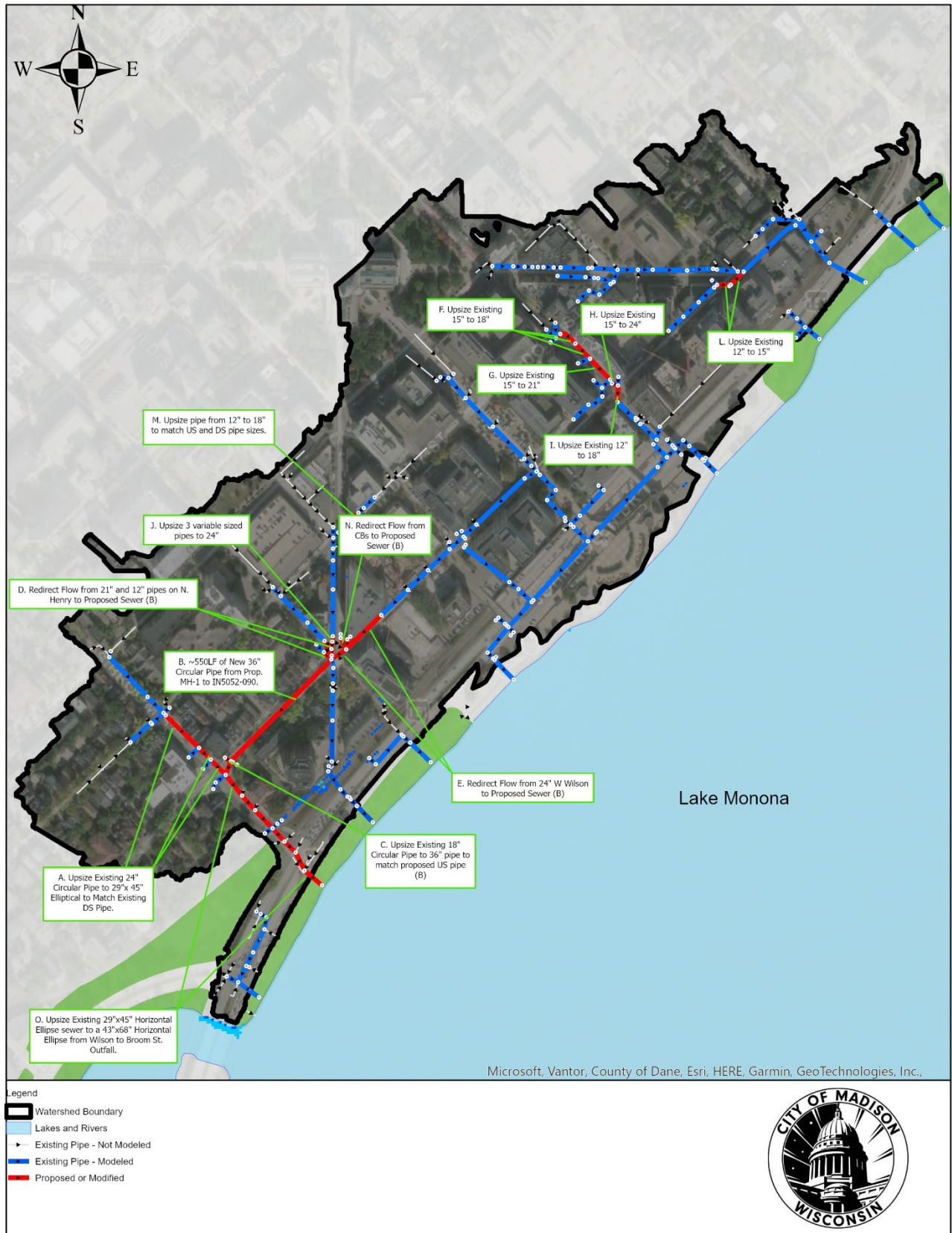
Figure ES-2: Alternative 3 – Schematic (Chosen Alternative)
