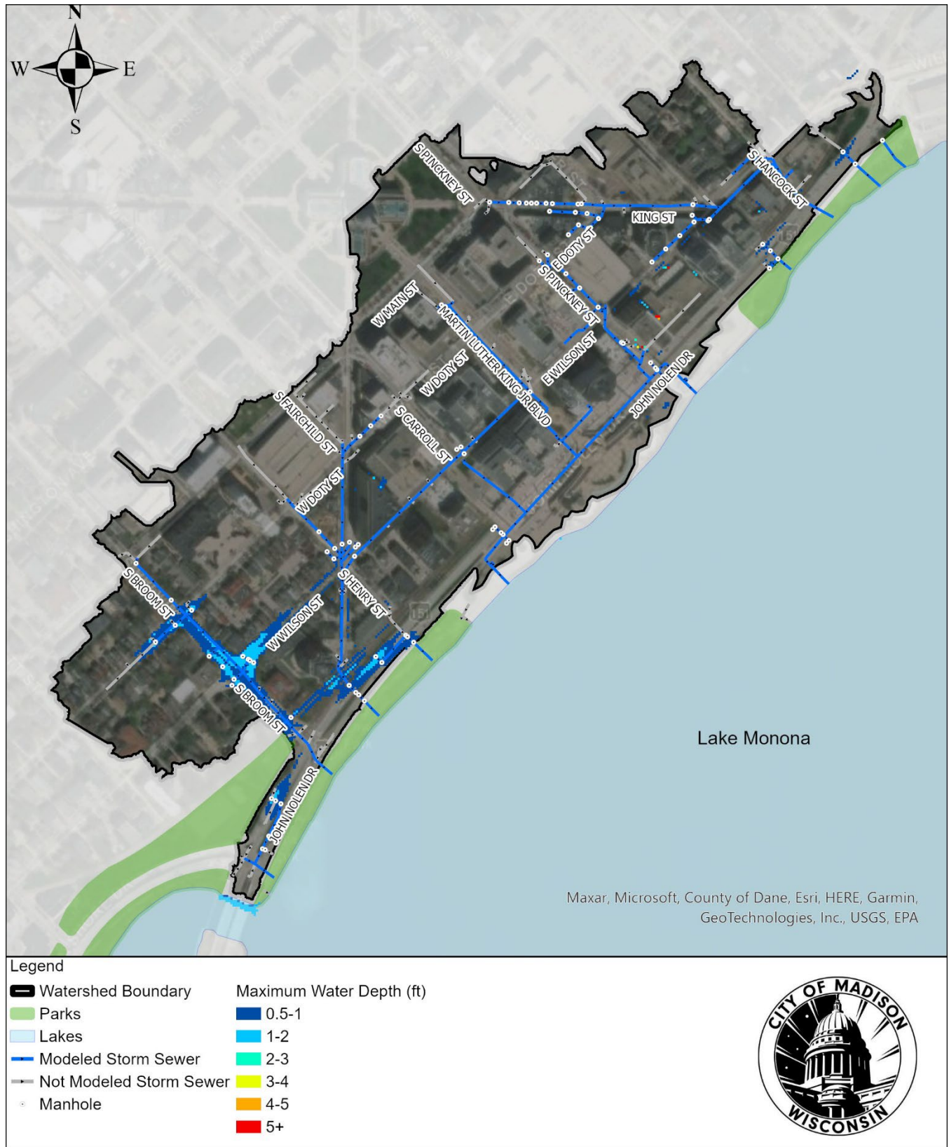
Figure 6-4: Projected Existing Condition Flooding During 0.2 percent AEP Design Storm
