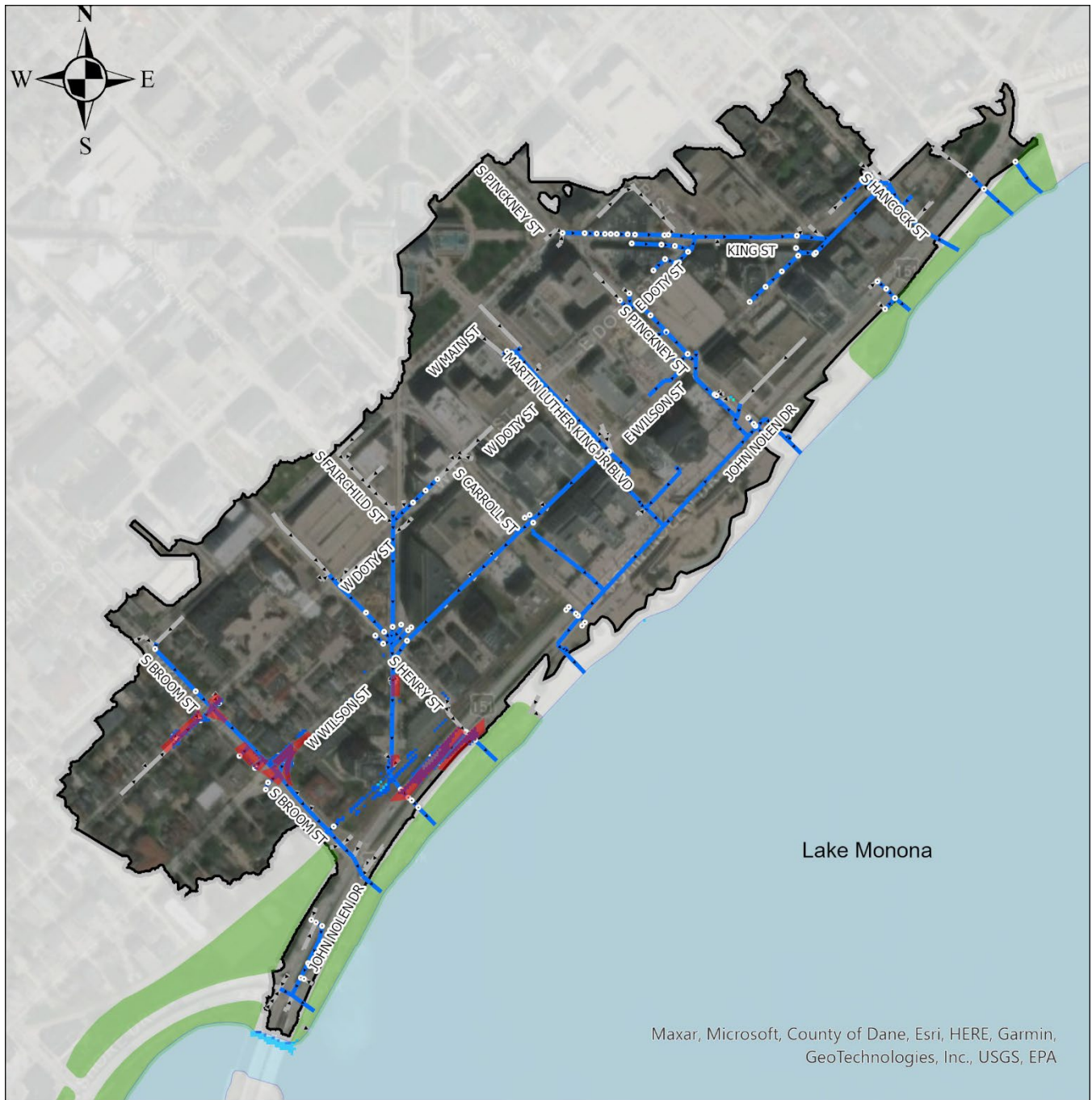
Figure 6-2: Projected Existing Condition Non-Drivable Streets during 4 percent AEP Design Storm
