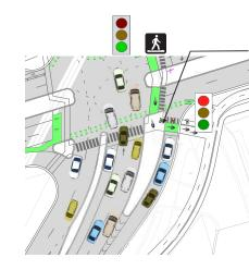
The channelization of the right turns allow the right turn lane to be controlled independently of the through lanes and walk signal. So the 900 vehicles and the 200 pedestrians/cyclist each have a separate signal phase.
