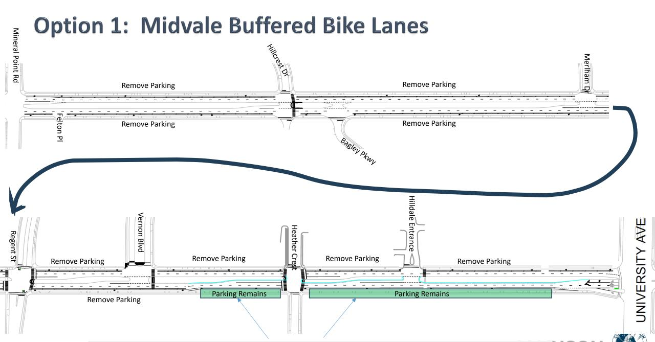
Green = Location where the center median narrowed to allow both parking and a bike lane
