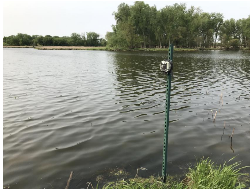
Above: Warner Lagoon Water Level Meter Left: Rain Gauge
