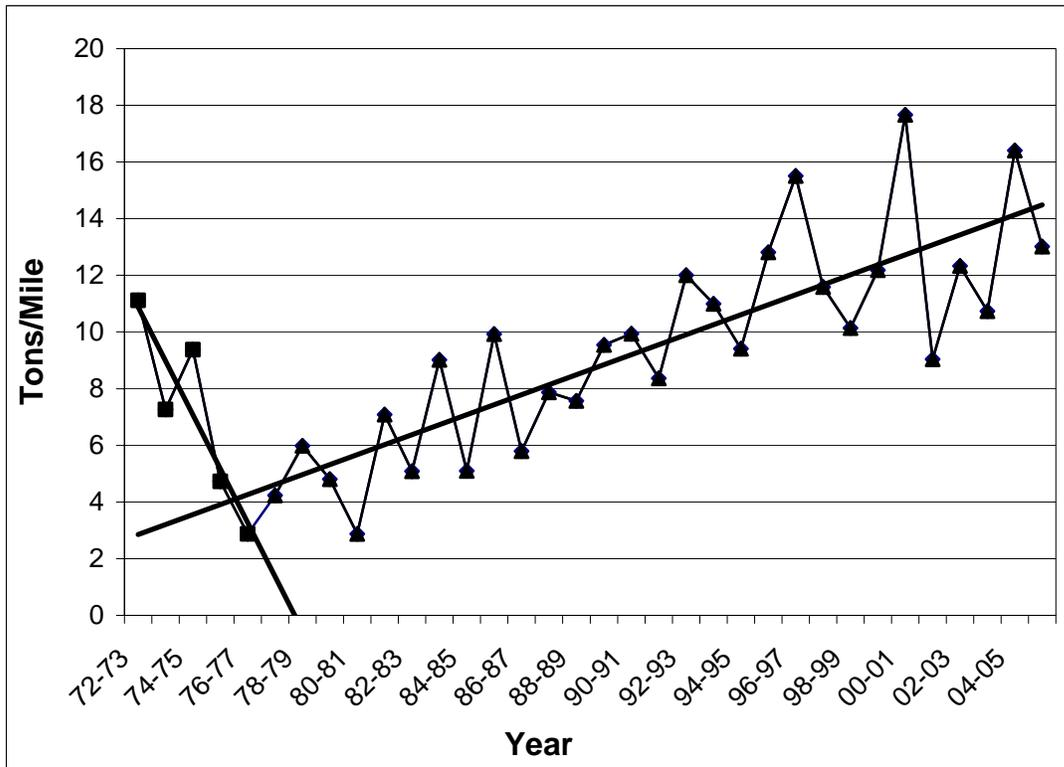
**Figure 4: Salt Use Per Mile of Maintained Street** (The scatter of the points above and below the line is, in large part, due to the variation in the “severity” of the winter weather from year to year. The “street miles” used are the total miles of streets maintained by the City of Madison and not the street miles that are actually salted each winter.)
