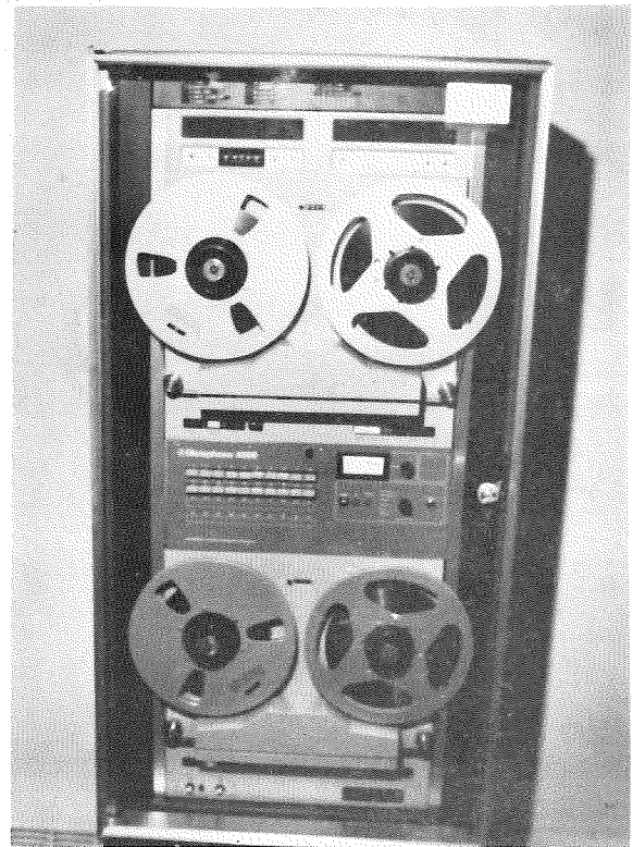
RECORDERS operate 24 hours a day, maintaining an electronic record of all emergency telephone and radio transmissions.
