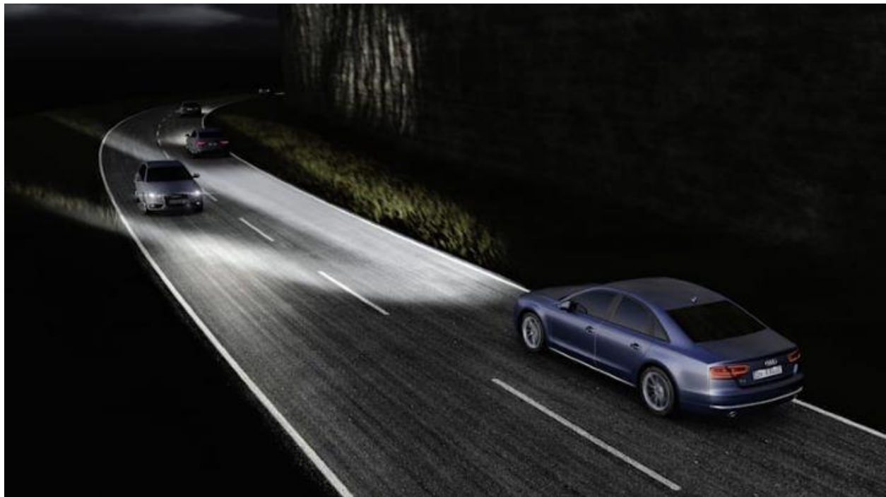
Figure 43. Artist rendering of Audi adaptive headlight beam technology 36
