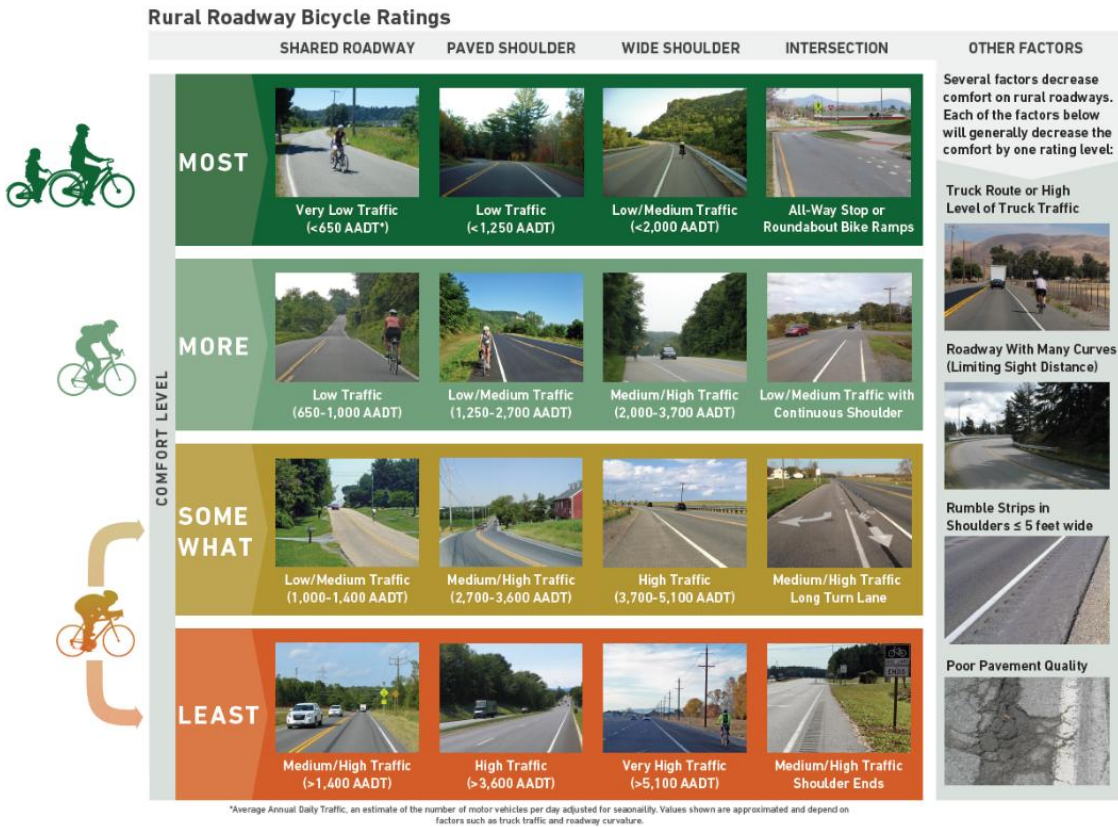
Figure 50-49. Rural Roadway Bicycle Ratings
