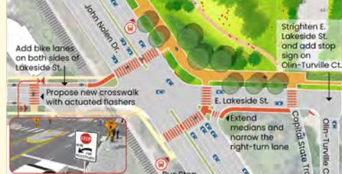
reduce curb radii to slow traffic and shorten crossings, and limit right-turns on red. Sasaki will work with the City Engineer to evaluate and develop these concepts.
