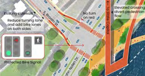
comprehensively enhance bike and pedestrian crossings to the lakefront paths, extend medians to provide physical protection for pedestrian crossings, make use of protected bike signals,
