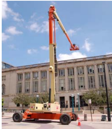
Figure 18 – Boom Lift used for Onsite Survey
