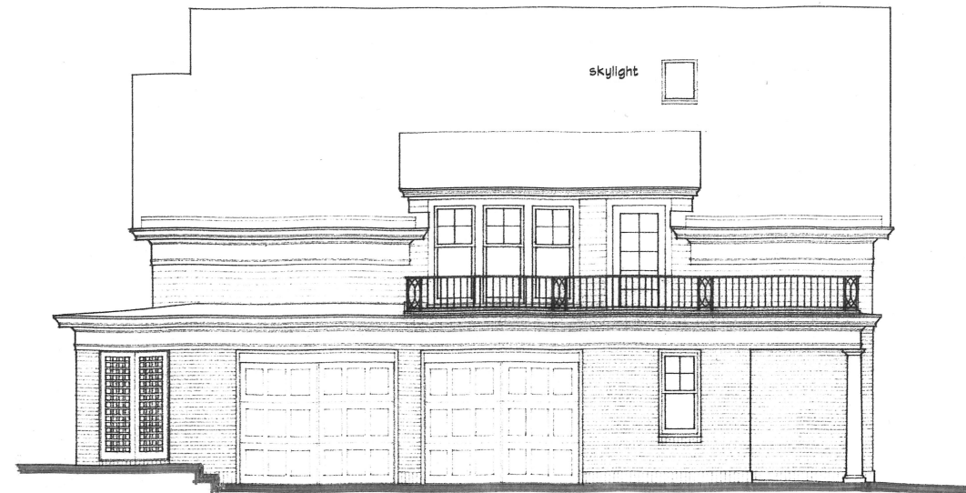
GARAGE/ADU NORTH ELEVATION
