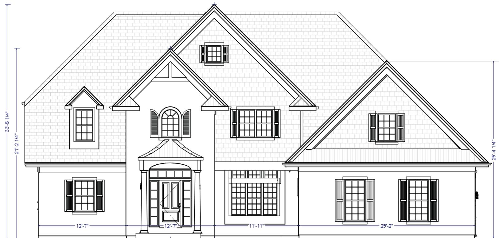
EXTERIOR MATERIALS: Natural cementitious stucco. Cedar shakes. Painted wood shutters. Asphalt shingles. Metal roof at entry. Painted LP SmartTrim (or equiv).
