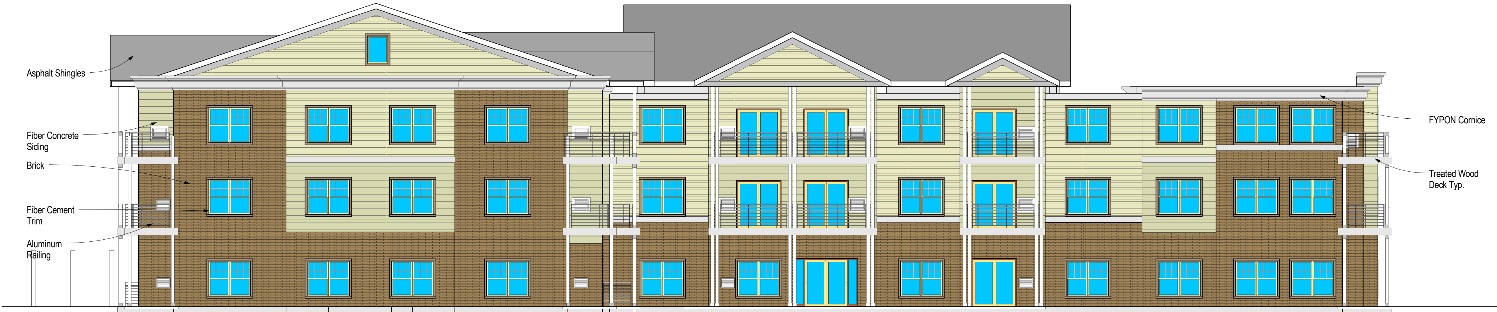
1 East Elevation - Sloped Roof Option 1/8" = 1'-0"
