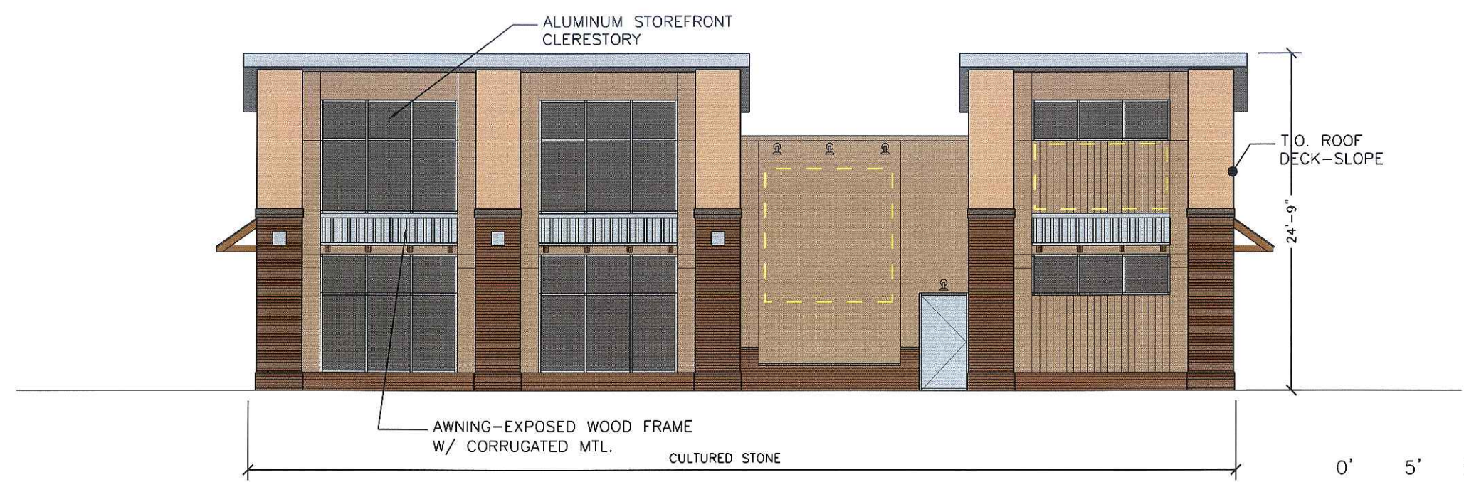
EAST ELEVATION ENTRY DRIVE ELEVATION
