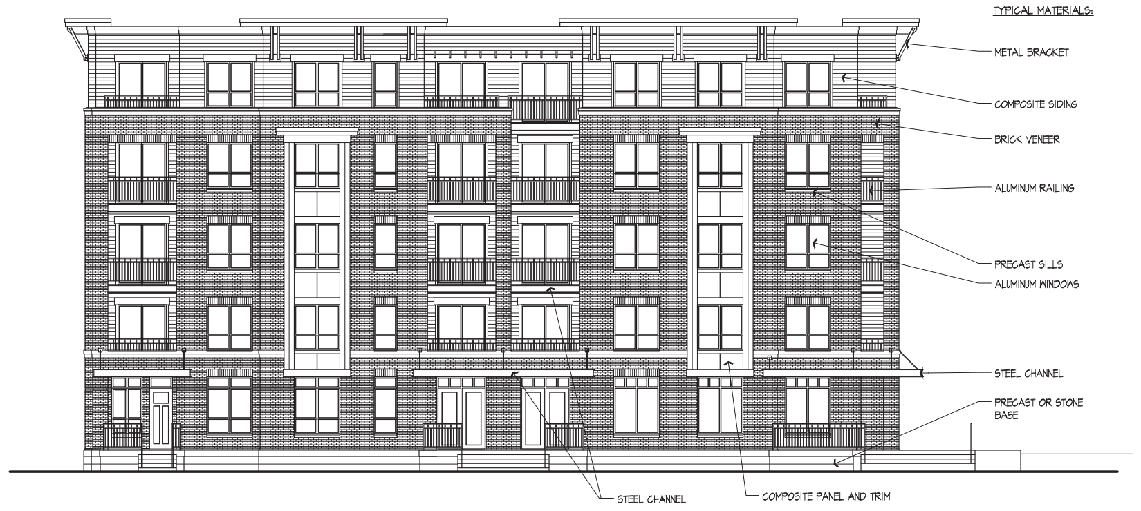
Bassett Street Elevation 1/8" = 1'-0"
